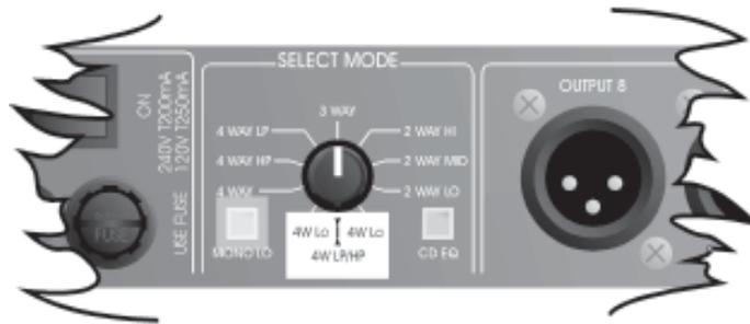
The MONO LOW switch operates in all stereo modes of operation and actively sums the signal information together on the LOW outputs. Both left and right LOW outputs will then contain the summed LOW signal.
