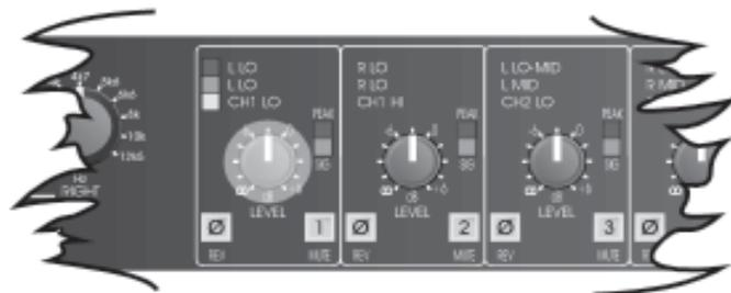
Individual output control adjustable from -6dB of gain to OFF. To ensure adequate resolution, the first 12dB of control range covers approximately 60% of the available control rotation.
