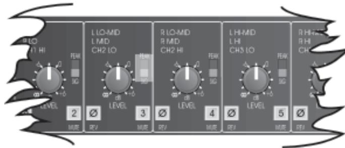
The SIG LED indicated that a signal is being received within that band, and the PEAK LED warns of the possible onset of system overload. The SIG LED will not light for signals below peak level of -20dB, and the PEAK LED lights for signals in excess of +10dB. This does not represent the maximum signal level within the **FDS-318** (which is +20dBv), but rather that the sound system is being driven very hard. For a more detailed explanation of this, **refer to section 11.6.**
