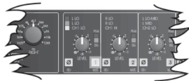
Push to MUTE the signal in the selected band. The number marked on the switch cap corresponds to the numbered output connectors on the rear panel.
