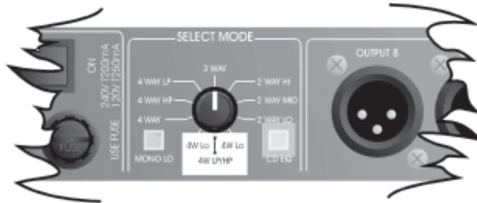
The CD EQ switch inserts constant directivity equalisation on all relevant outputs, dependant on the mode selected. **Refer to the table in section 11.1** for more information.
