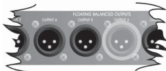
The outputs are electronically balanced and floating. Maximum output is +20dBu into 600 ohms or greater. Transformer balancing is NOT available as an internally fitted option, and so the BSS AR-204 balancing unit should be specified if required.
