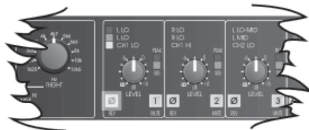
Individual polarity reverse selector switch. Push to invert the polarity of the signal in that band.
