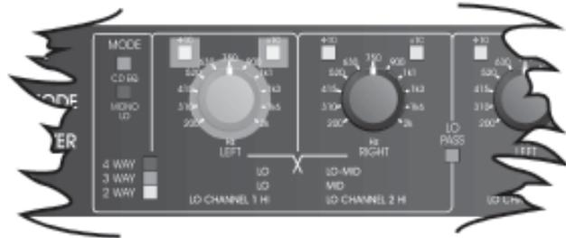
Left and right hand channels are adjustable separately. The frequency scaling LEDs, marked as x10 and /10, indicates whether the printed frequency scale needs to be multiplied or divided by 10 for the correct value. The control of this is determined by the SELECT MODE switch on the rear panel.
