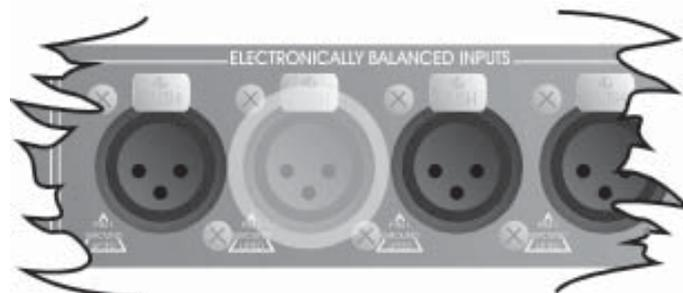
The inputs are electronically balanced. Maximum input is +20dBu in to 10Kohms. Transformer balancing is NOT available as an internally fitted option. Inputs 1 and 2 are used for the 4- and 3-way modes. Inputs 1, 2, 3 and 4 are used for the 2-way modes.
