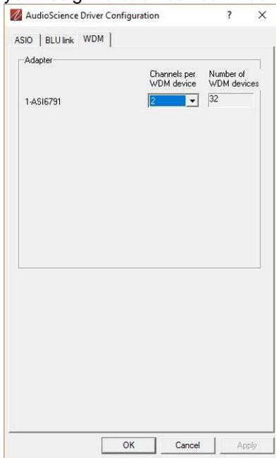
The “Channels per WDM device” drop down allows you to change the number of channels assigned to each WDM device in Windows. Changing this value will update the “Number of WDM devices” information box where you will be able to see the number of devices you will get based on your chosen channel value. The values assigned here will apply to both the WDM and ASIO drivers.
