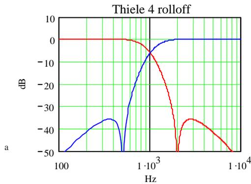
An NTM™ Crossover Filter sums precisely to give constant output and well defined phase response, which is identical between the drivers (zero degrees difference) throughout the crossover region.
