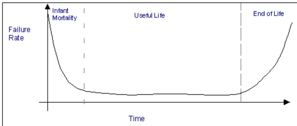
Figure 1 – The “Bathtub” Curve<sup>ii</sup>
