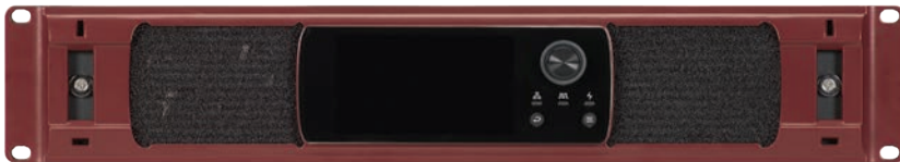
Figure 3a: Front plate removed to access air filters
