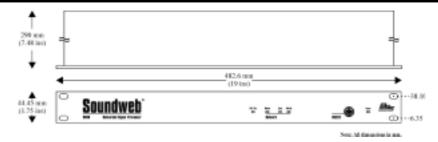
If the unit is likely to undergo extreme vibration through extensive road trucking and touring, it must be supported at the rear and/or sides to lessen the stress on the front mounting flange. Use either a ready-built rack tray or mount the 9008 unit between other units. Damage caused by insufficient support is not covered by the warranty.
